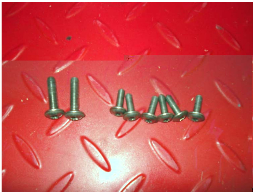
Lower Panel screws – the 2 T-27's are on the left.
