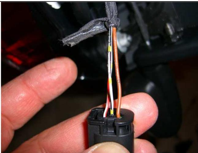
On GS models, remove the tail light mounting from the motorcycle to gain access to the electrical plug. Strip back two inches of protective wire tape to expose the wires. The center GR/SW/GE wire possesses both brake & tail signals, so this is the wire to connect the trigger lead from the harness for the can bus brake-tail light.
