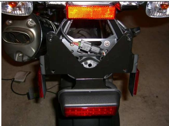
Secure the can bus brake-tail light to the license plate holder, and then secure the plug connection to the frame to ensure it does not become damaged.
