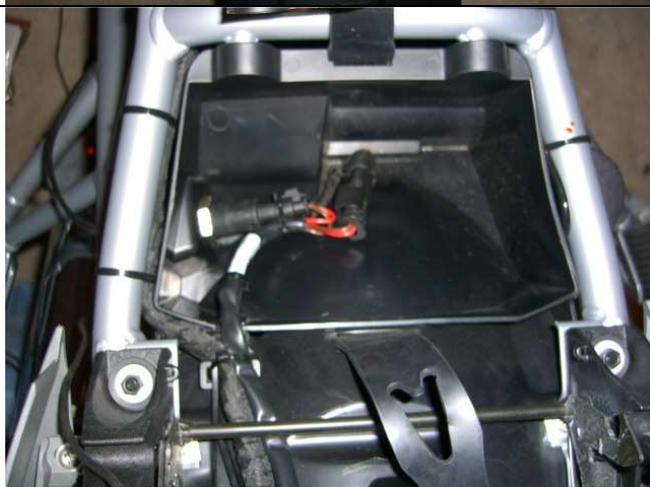
Run the can bus brake-tail light harness beside the factory harness from the tail light area to the power accessory outlet. Secure with cable ties and plug into the accessory outlet with the special Hirschman pin and socket housings supplied with the harness. Secure with cable ties as shown.
