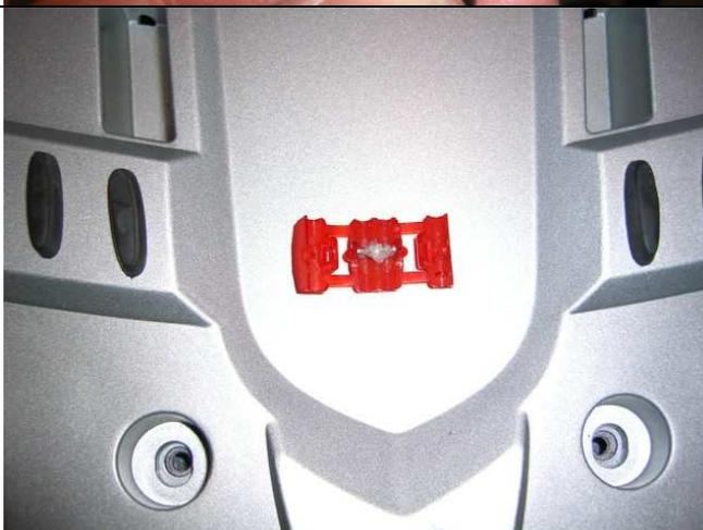
Apply a small amount of die-electric grease to the connector to prevent corrosion later in use. Cut-off the 1/4" male/female blade connector from the trigger wire, strip back the PVC cover 1.5" to enable connection to the splice connector. Connect the GR/SW/GE wire to this connector, and then install the trigger wire from the harness.
